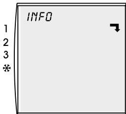
When this arrow appears on the display, a submenu is available. Press the right-hand setting knob (menu) again to open this submenu.
