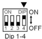
These dipswitches are set correctly ex factory and they do not have to be adjusted. Refer to the picture for a correct setting of the dipswitches; if they are set incorrectly, the room thermostat will not work!
