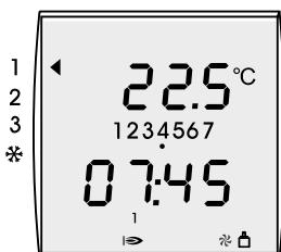
The display briefly shows all available functions; subsequently, the software version is displayed during 3 seconds.
