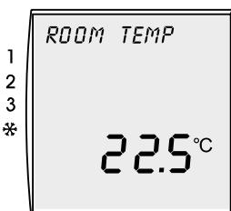
With the key **Info** you can call up the set room temperature, the current room temperature and, if an outdoor sensor is connected to the air heater, also the outdoor temperature.
